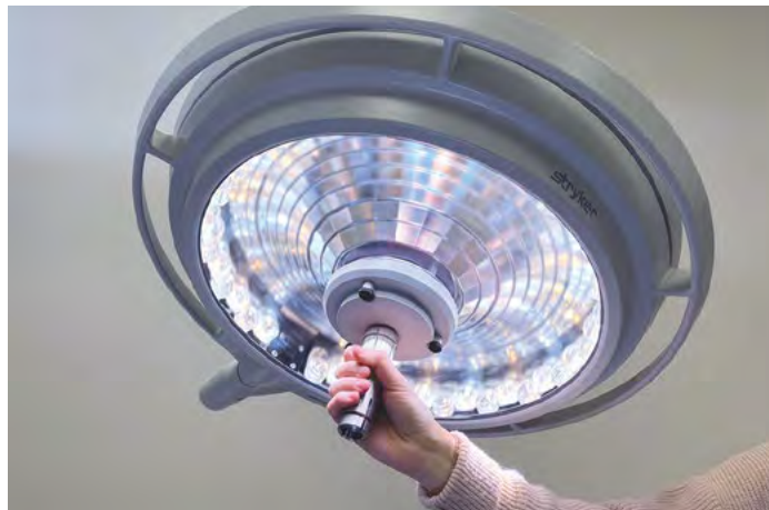
The new surgical lights are adjustable by a handle or a wall-mounted digital panel.
